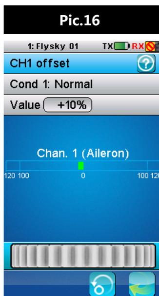
This function can be used to correct problems with alignment. For example if a servos range of motion is too great in one direction and not enough in another, it is possible to offset the channel by +/- 50%.
