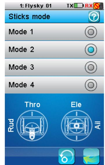
Changing from modes 2/4 to 1/3 will change the throttle position. This will require the user to open the system and switch the stick positions. The gimbals can be switched by following these instructions.
