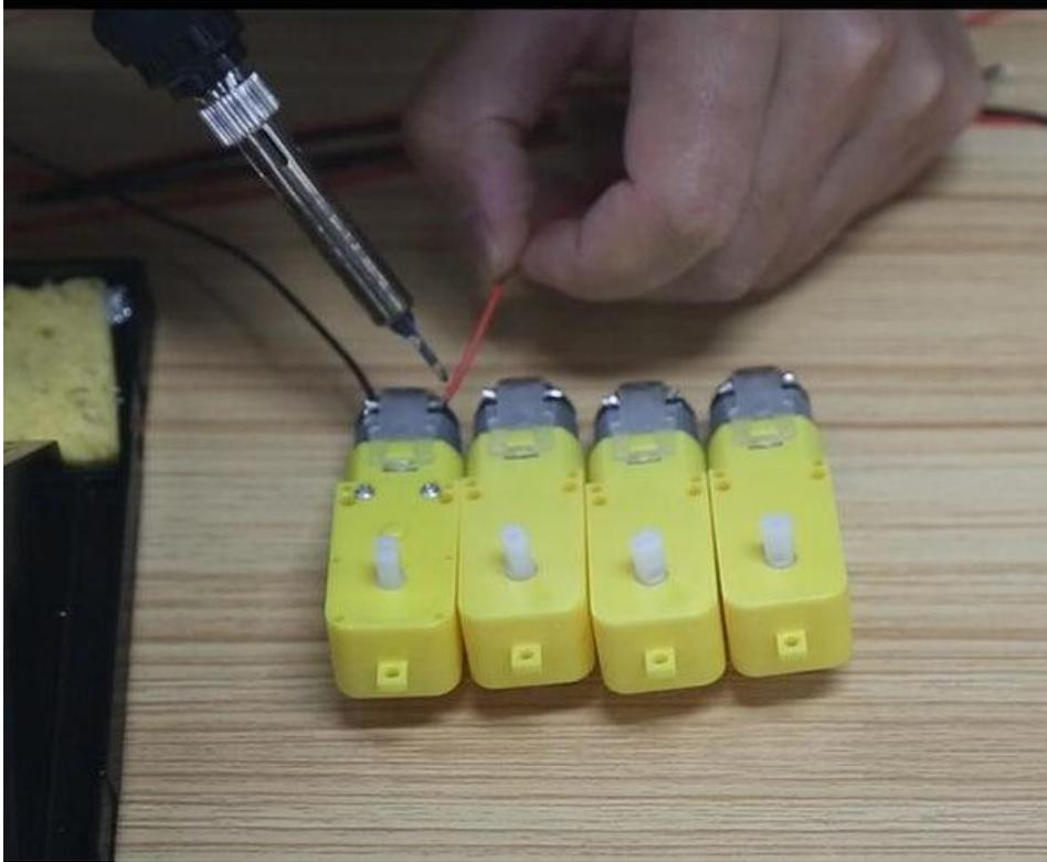
After soldering, connect the fixing post of the motor to the motor with long screws and nuts.
