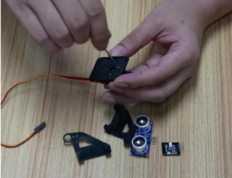
Install the brackets on the left and right sides of the servo, align the raised positions of the servo, and use two screws to fix the sides of the bracket.
